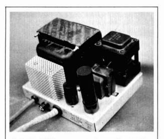
The Collins 516F-2 power supply after modification. The silicon replacement rectifiers substitute for the rectifier tubes.
